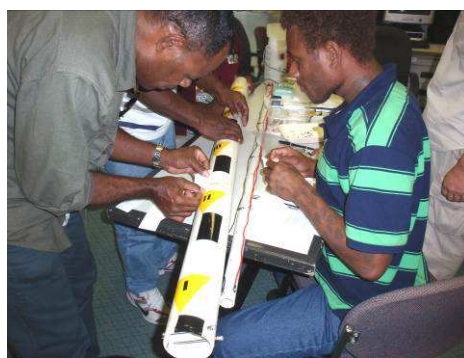
Assembly of Stream gage (Fiji 2011)
