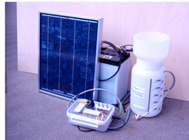
Complete set of rain gage with solar panel and battery
