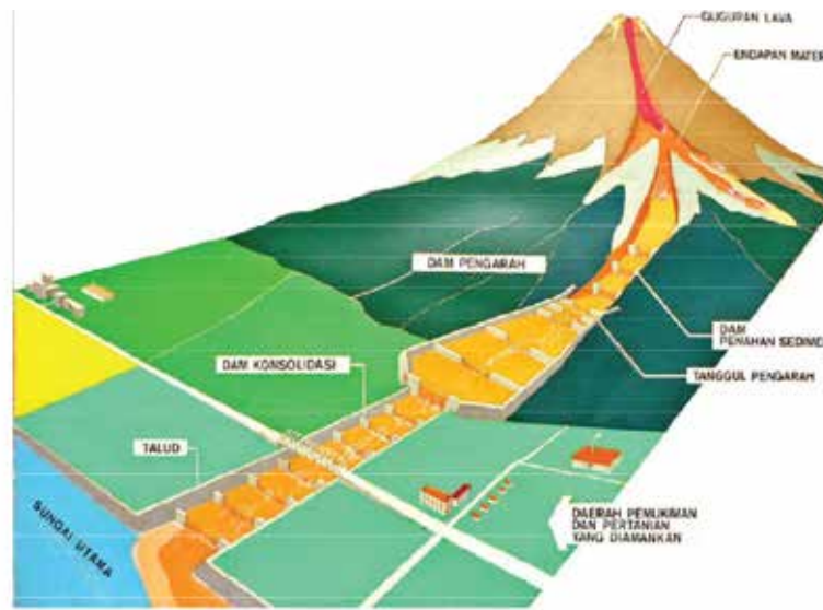
Figure 22: Debris Flow Control Model
