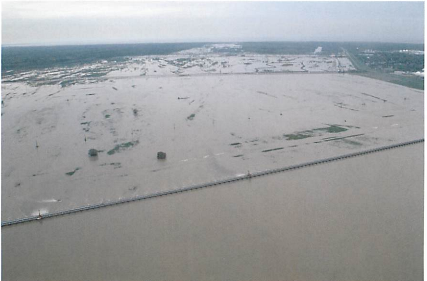
Map of Bonnet Carré Spillway (top), and aerial of the spillway in operation during the flood of 1975. The view is from the Mississippi River with Lake Pontchartrain in the background.
