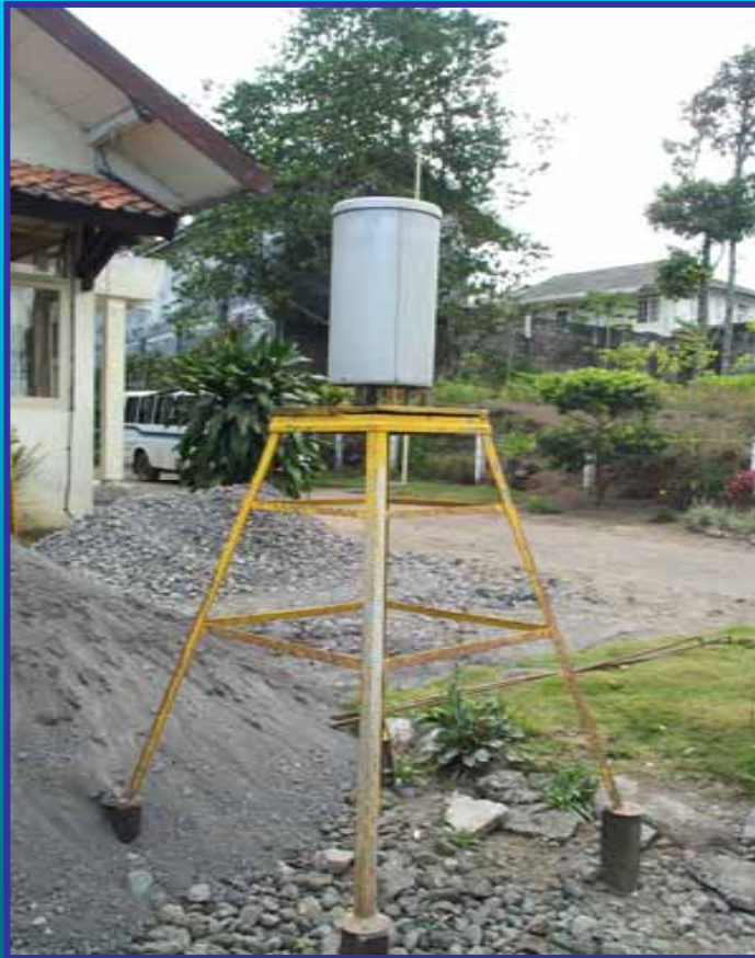
Automatic rain gauge in Kaliurang
