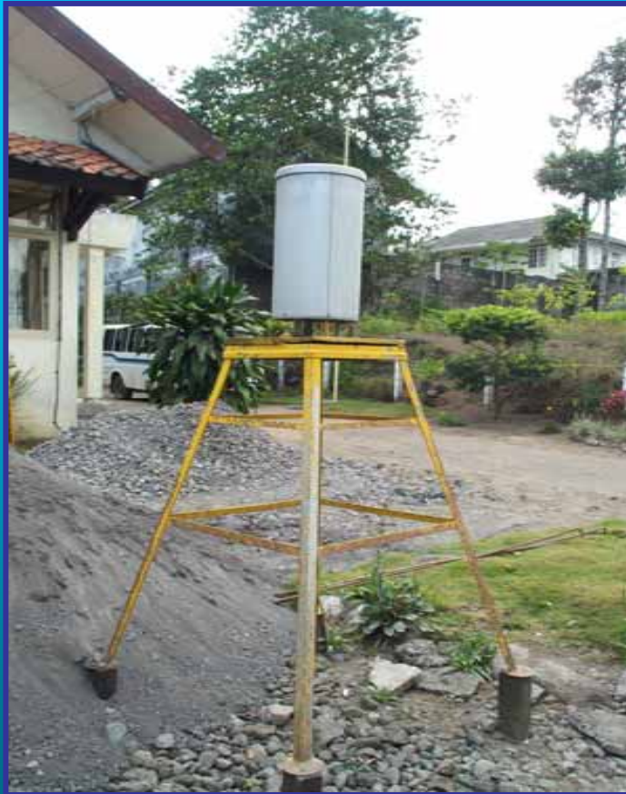
Automatic rain gauge in Kaliurang
