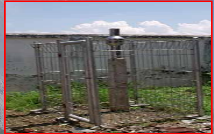
Non-telemeter Automatic Rain Gauge in Mujur River Catchment Area
