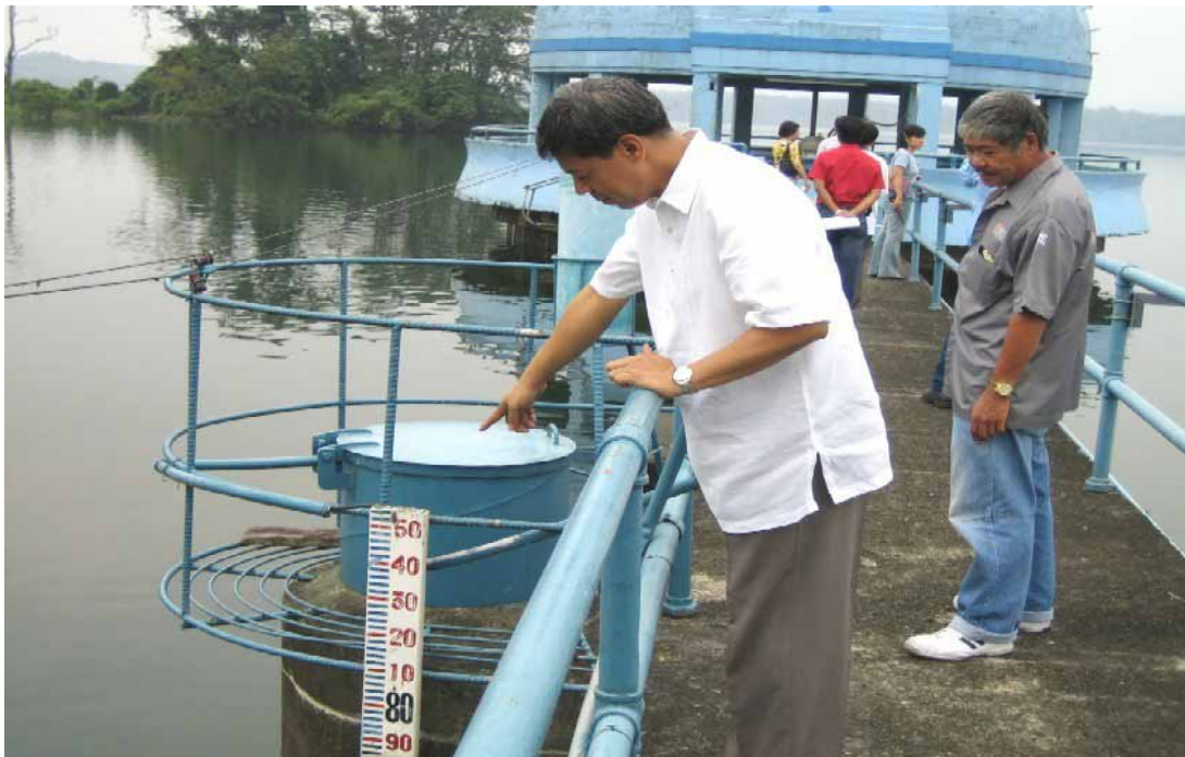
A SCALE FOR MEASURING THE WATER LEVEL OF THE DAM, BEFORE REACHING THE CRITICAL LEVEL, RESIDENTS OF ODELCO COMPOUND AND CALIFORNIA RIVERSIDE IN SAN BARTOLOME NEED TO BE INFORMED
