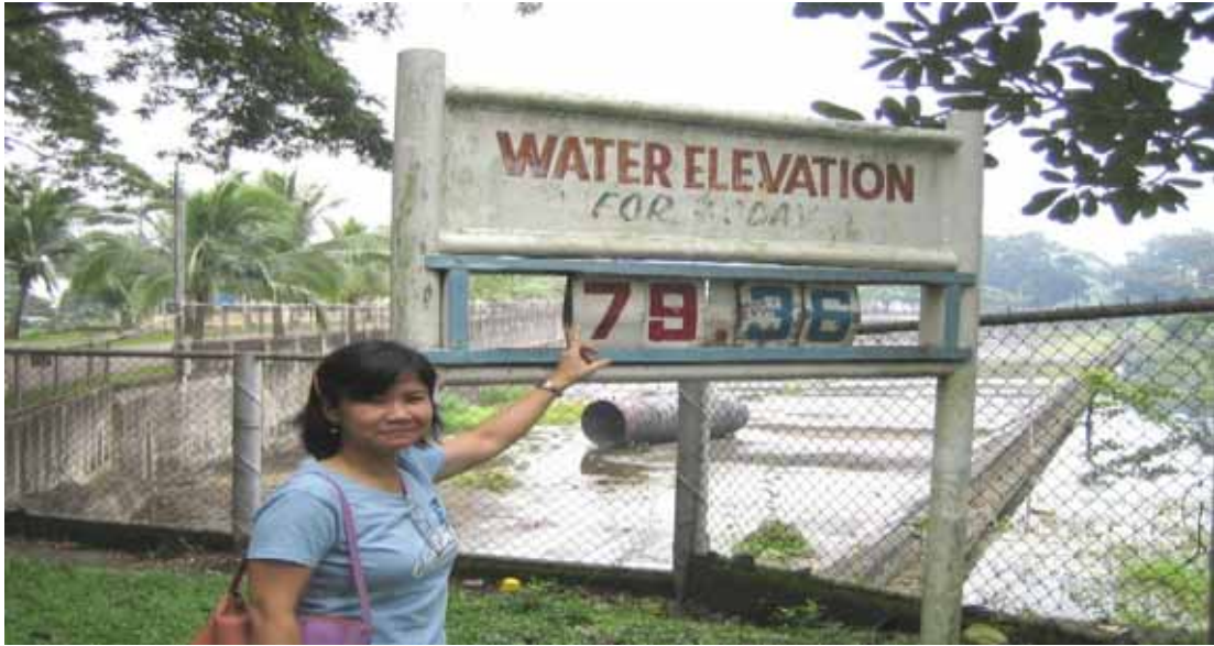
A SIGNBOARD FOR MONITORING THE WATER LEVEL SO THAT RESIDENT MAY KNOW, ALSO SERVE AS A WARNING DEVICE FOR EVACUATION PURPOSES
